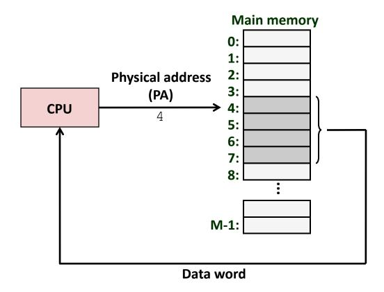
Used in some "simple" systems, like embedded microcontrollers in cars, elevators, and digital picture frames
