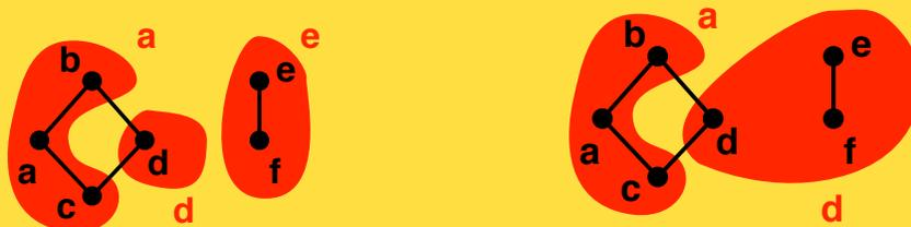
*The partitioning on the left is appropriate for graph contraction since each partition is connected. The partitioning on the right is not since  $d$  is not connected to  $e$  and  $f$ .*
