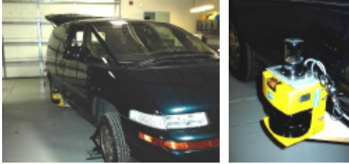
Fig. 15: Navlab8, SICK PLS100, and an omni-directional camera.
