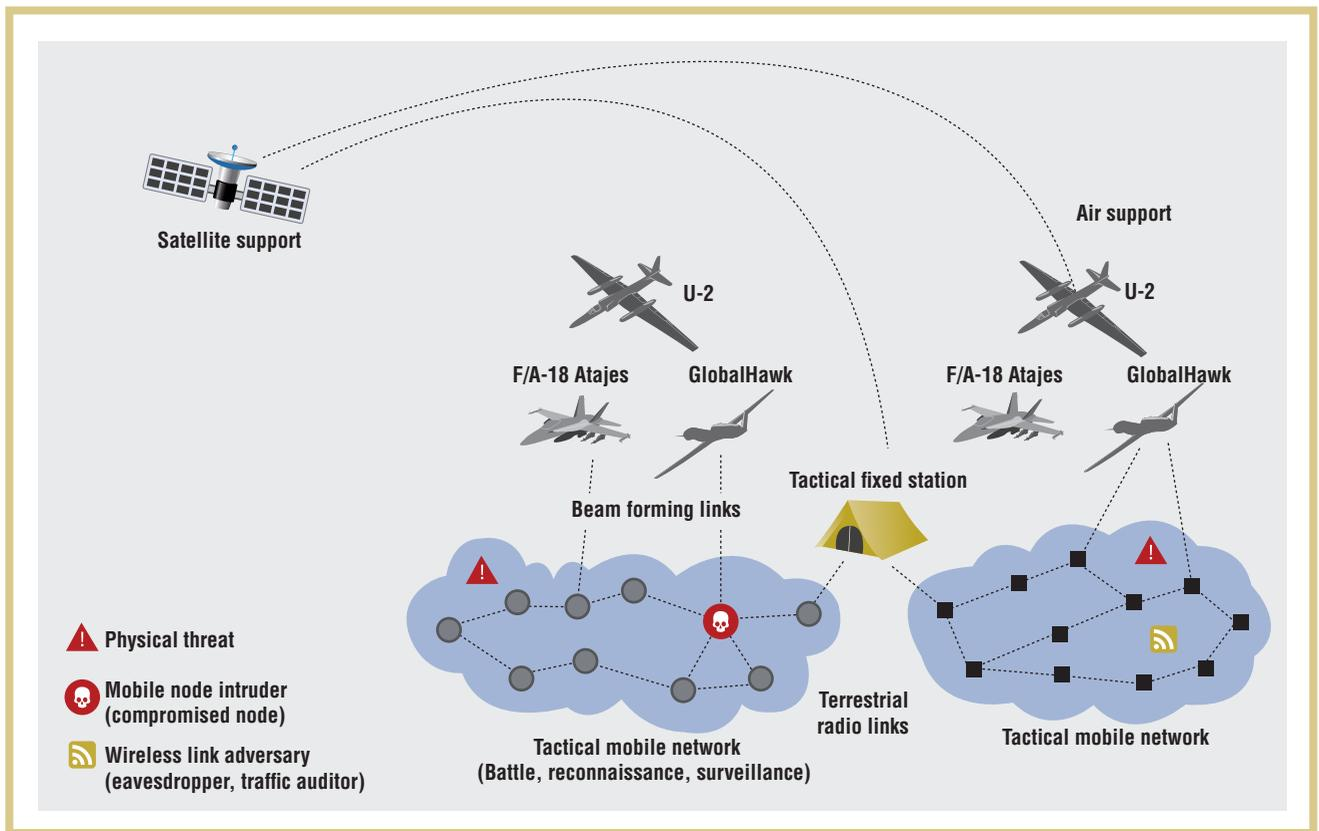
Figure 1. An example combat network.<sup>9</sup> The wide-area links based on satellite and air support are the most vulnerable to wireless jamming attacks from a distance.
