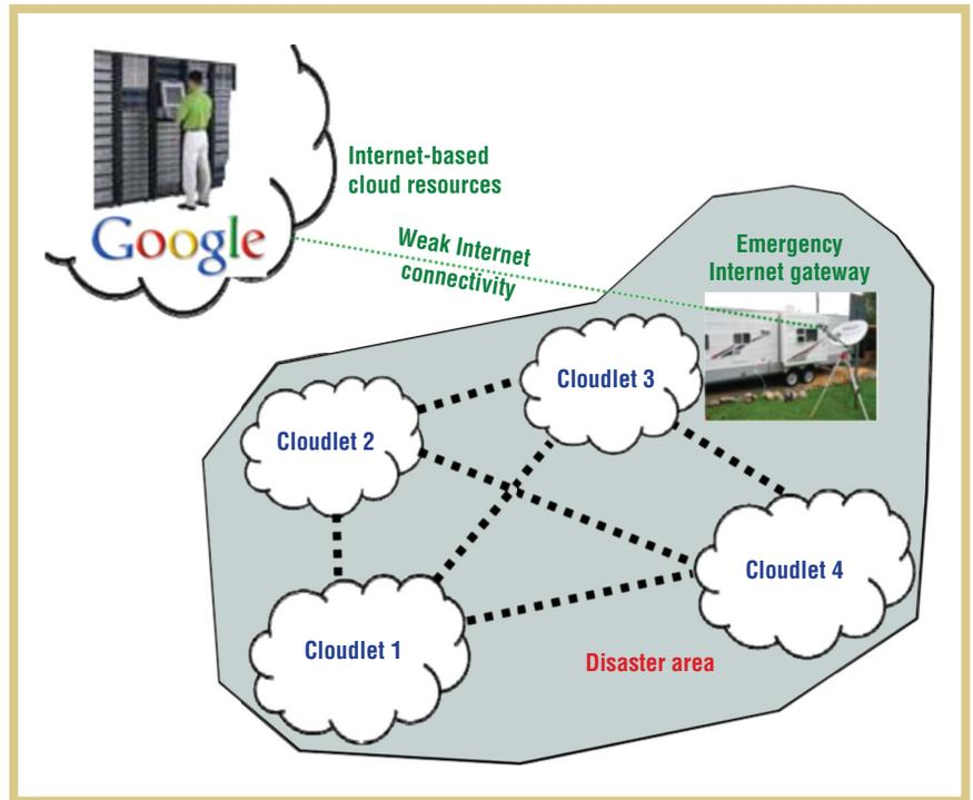
Figure 3. A cloudlet ensemble. An ensemble of cloudlets with mesh connectivity can offer reliable cloud computing services within a disaster recovery area even with a fragile backhaul to the cloud.
