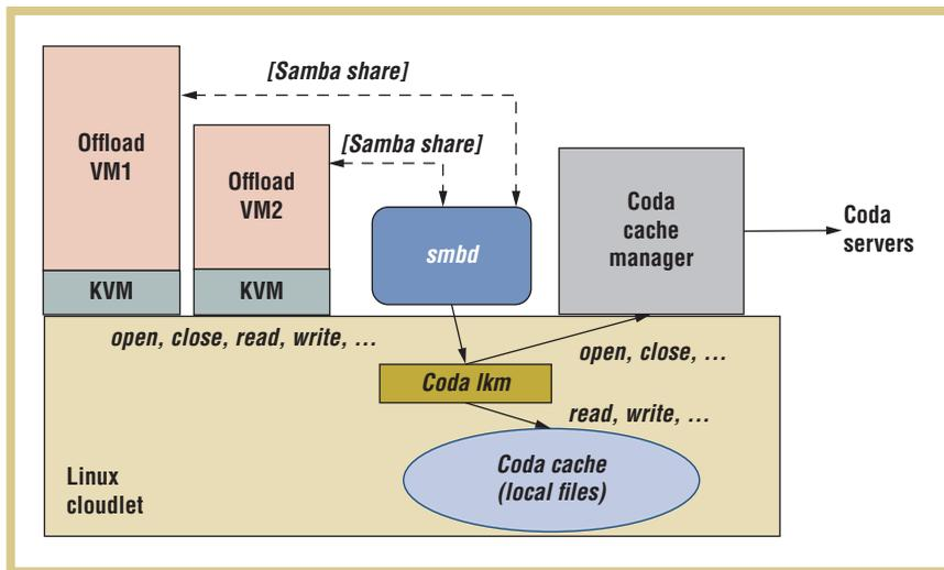
Figure 4. Virtual machine access to shared data. This offers strong file system consistency for offload operations.
