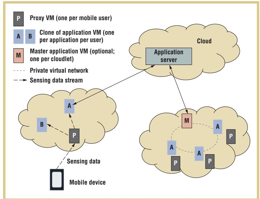
Figure 5. Proxy VMs in cloudlets.<sup>16</sup> The proxy VM mediates all interactions by the mobile device with other mobile devices or with cloud/cloudlet services.
