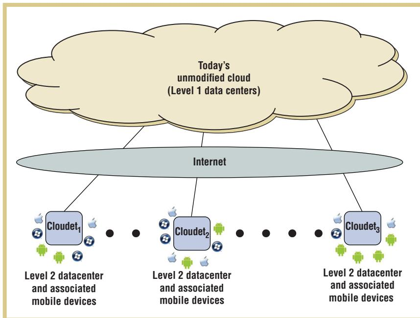
Figure 2. A two-level cloud computing architecture. Level 1 is today's unmodified cloud infrastructure, and level 2 comprises cloudlets that are dynamically associated with nearby mobile devices.
