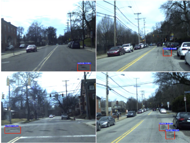
Figure 5: Examples of pothole detections with bounding boxes.
