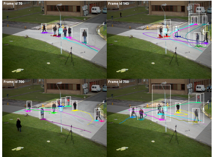
Fig. 3: Tracking results of MOTIS on the PETS2009 S2L1 dataset. A video showing the whole results is available at http://goo.gl/4QIIey .
