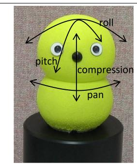
Figure 3. The four axes of the Keepon robot
