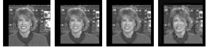
A. Original Image B. Reconstruction from projection of A. MSE = 165.6 C. Reconstruction from sparse coded version of A. MSE = 179.2 D. Reconstruction from quantized version of A. MSE = 295.8.
