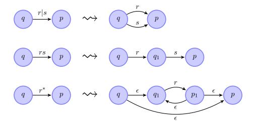
When applying the rule we match on the pattern on the left in the current candidate for an NFA and replace it by the right, introducing new states  $q_1$ ,  $q_2$  as necessary.
