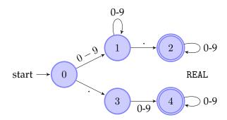
Of course, when we use this finite automaton to recognize the number 3.1415926 in the input stream 3.1415926-3+x;if, then we do not only want to know that a token of type REAL has been recognized and that the remaining input is -3+x;if. We also want to know what the value of the token of type REAL has been, so we store it's value along with the token type.
