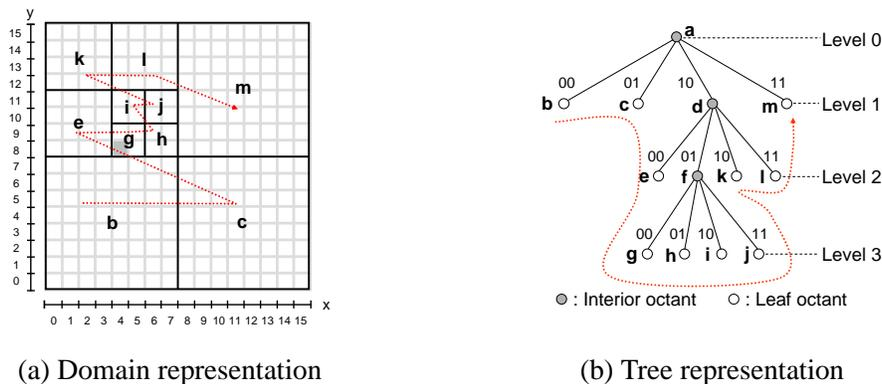
Figure 3: **Equivalent representations of an octree.**
