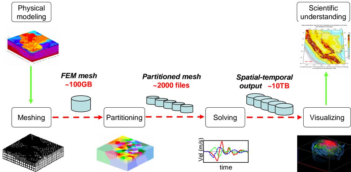
Figure 1: **Traditional simulation pipeline.**
