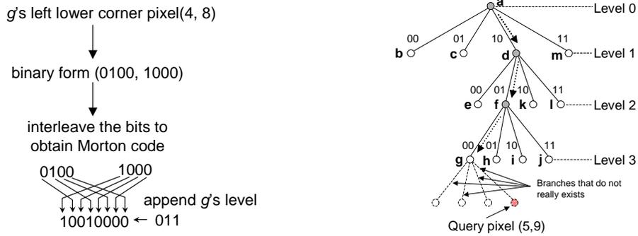
(a) Computing the locational code for  $g$ . (b) Aggregate hit of a pixel in an octant.
