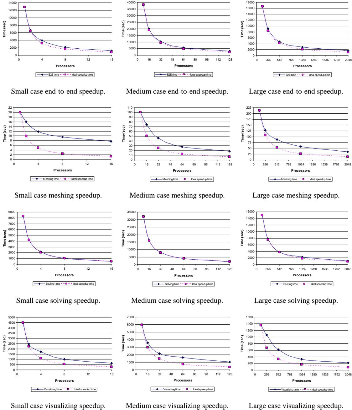
Figure 14: **Speedups of fixed-size experiments.** The first row represents the end-to-end running time; the second the meshing and partitioning time; the third the solving time; and the fourth the visualizing time.
