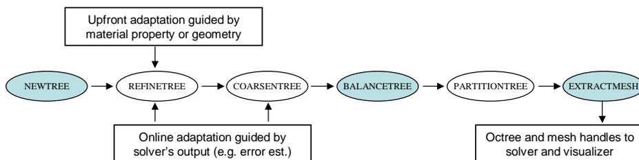
Figure 7: **Meshing component.** Shaded ovals are required steps. Unshaded ovals are optional steps.
