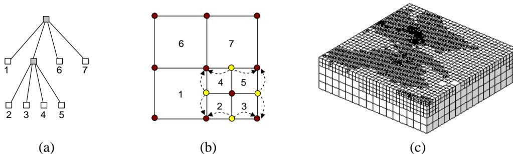
Figure 6: **Octree-based hexahedral meshes.** (a) Octree domain decomposition. (b) Octants map to elements and vertices map to mesh nodes. The dark colored dots represent the anchored nodes and the light colored dots represent the dangling nodes. The dashed arrows represent the explicit correlations between dangling nodes and anchored nodes. (c) An example 3D octree mesh.
