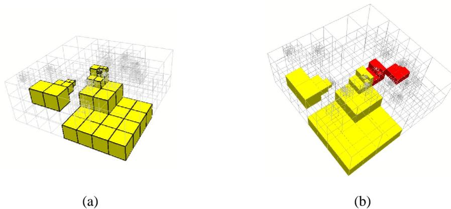
Figure 15: **Workload distribution.** (a) Elements assigned on one processor. (b) Unbalanced visualization workload on two processors.
