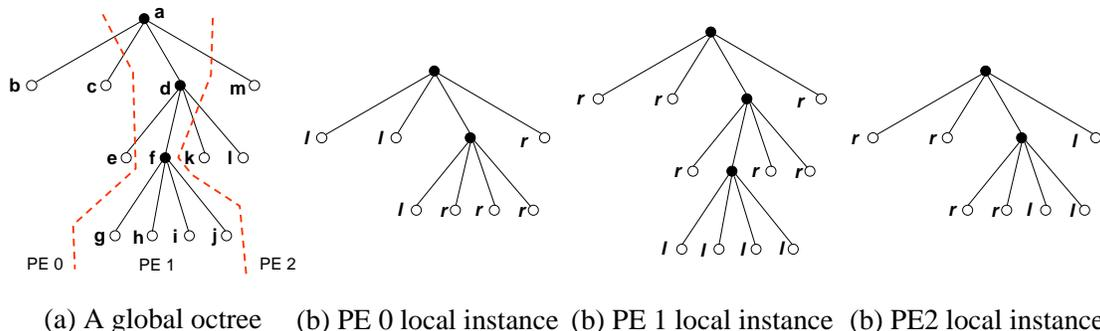
Figure 5: **Parallel octree organization on 3 processors.** Circles marked by 1 represent local leaf octants; and those marked by r represent aggregated remote leaf octants.
