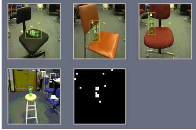
Figure 2: Detection of a bottle from previous examples. The top row contains images where the outlined part contains the tiles used as positive examples. The rest of the image's tiles are negative examples. Probabilities above 0.8 are marked in the previously unseen picture in the bottom row. Not shown is another set of 18 “background” pictures consisting of negative examples only.
