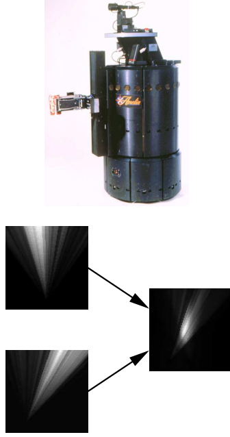
Figure 3: On the top, the robot used in our experiments is shown. It is equipped with a parallel two-fingered gripper for object manipulation. On the bottom, an illustration is presented of how information from images taken from two different viewpoint is integrated in the occupancy grid. Shown to the left are two single projections applied to an “empty” grid. The picture on the right shows how they are combined together. The images depict the average values of grid cell probabilities when viewed from above (i.e. averaging probability values along the z -axis).
