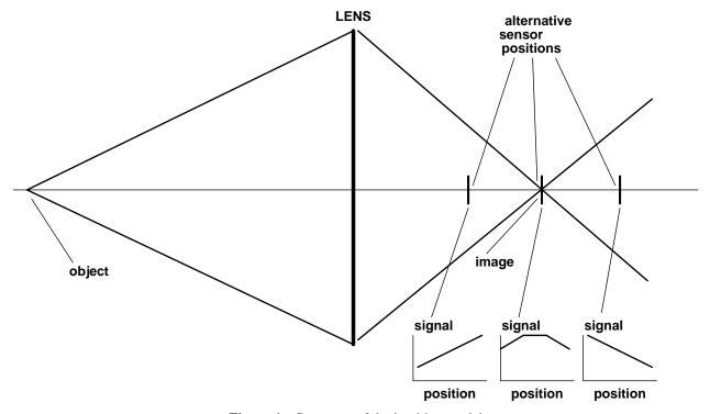
**Figure 1:** Geometry of the intuitive model
