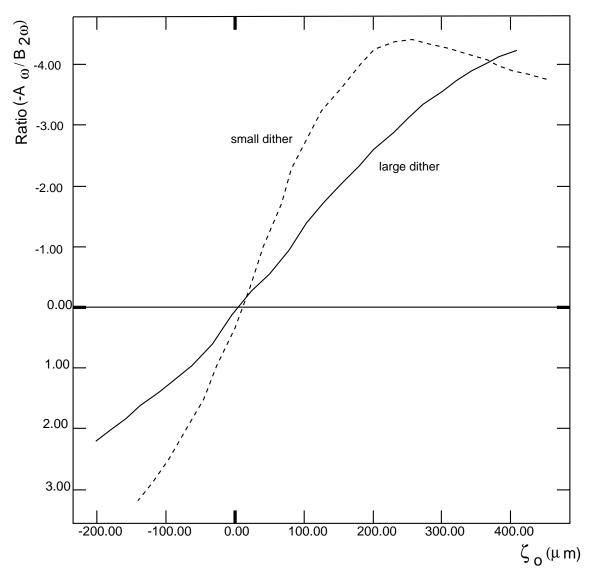
**Figure 4:** Dither amplitude vs dynamic range
