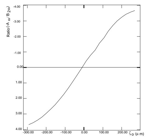
Figure 2: Ratio of first harmonic to second harmonic vs focus error
