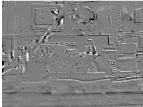
(e) Error in the synthesized intermediate view using FBS-DCP disparity map (PSNR=23.3dB) [(a) - (g)]
