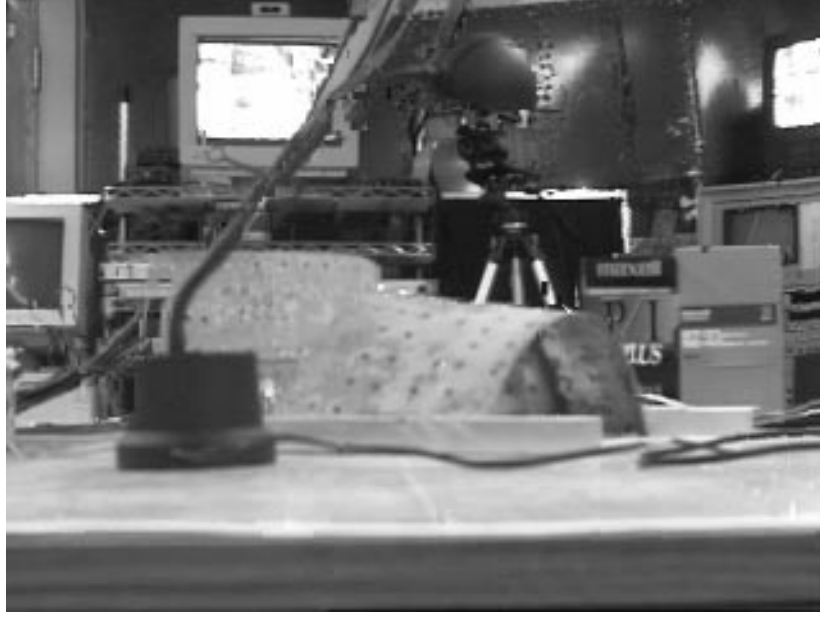
(f) Intermediate view (for \alpha=0.5 ) synthesized using the DBS disparity map
