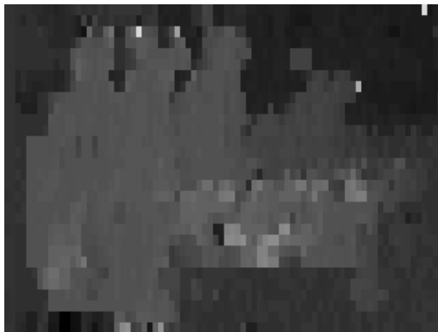
Fig. 3.6 (c) Disparity map obtained using FBS-based DCP with 8x8 blocks The smoothness of the map is affected by the spurious matches.
