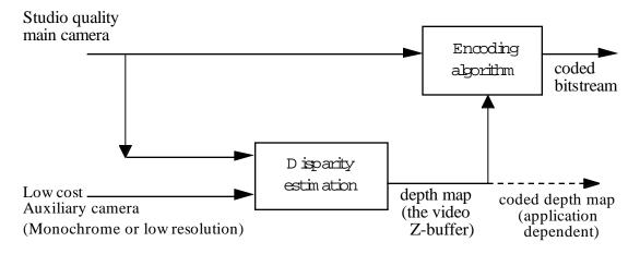
Fig. 1: Schematic of the proposed video Z-buffer based monoscopic image compression scheme
