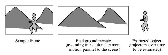
Fig. 2: (b) Nonstationary background identification and mosic construction
