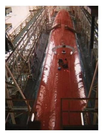
Fig. 5: CIMP on a 747 in a heavy maintenance bay at Northwest Airlines Minneapolis headquarters. The inspector, observed by a CMU staffer, is performing an eddy current check of a visual anomaly detected using the remote vision system shown in Fig. 7. Future models would incorporate remotely operated eddy current sensing.
