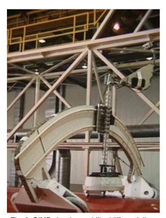
Fig. 6: CIMP showing mobility (differentially driven wheels), sensor pod mounted off circumference-scanning carriage, and wide angle cameras for navigation and proprioception or "self-awareness" (upper right). The vertical stalk and the sensor pod rotate to change the camera viewing azimuth. Curvature was designed for window-line to window-line access on a DC9.
