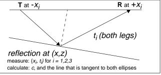
Fig. 6: Paths when layers are not of uniform thickness.
