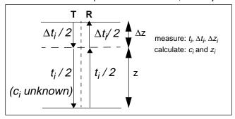
Fig. 2: Differential time-of-flight method.
