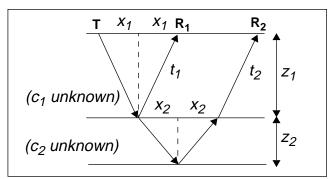
Fig. 4: Extending the method of Fig. 3 to multiple layers.
