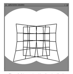
**Figure 9:** 2 lenses, pincushion distortion (E < 0) vertical disparity; cannot be fused
