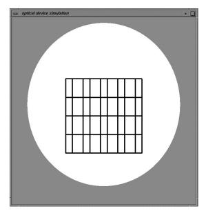
**Figure 3:** 1 lens, regular grid, no aberration; images: two 4×4 grids displaced left and right of center
