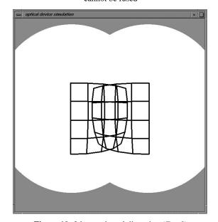
**Figure 10:** 2 lenses, barrel distortion (E > 0) vertical disparity; cannot be fused
