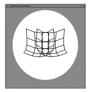
Figure 4: 1 lens, pure curvature-of-field ( $D \neq 0$ ) no vertical disparities; fuses into a curved surface as expected
