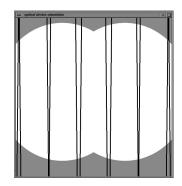
Figure 12: 2 lenses, vertical lines, pure curvature-of-field (D ≠ 0), vertical disparity is invisible; fuses into a curved surface
