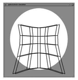
Figure 5: 1 lens, pincushion distortion (E < 0) no vertical disparity; fuses into a distorted but planar figure
