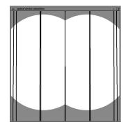
**Figure 13:** 2 lenses, vertical lines, barrel distortion (*E* < 0), vertical disparity is invisible; fuses into a curved surface
