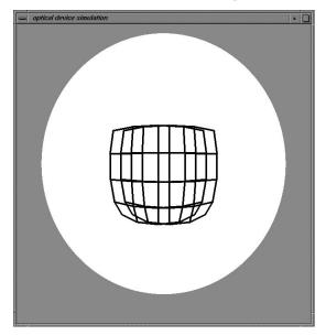
**Figure 6:** 1 lens, barrel distortion (E > 0) no vertical disparity; fuses into a distorted but planar figure
