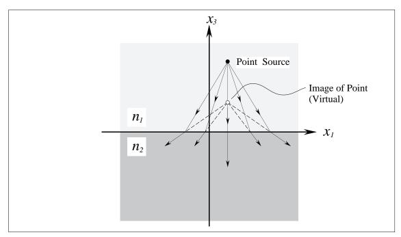
Figure 3. Flat interface between two media as an ideal optical device.
