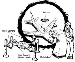
Figure 4. ROBOTIC AIRCRAFT INSPECTION CONCEPT
