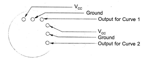
$V_{cc}$  should be controlled 5.00 volts. Output is ratiometric and depends on controlled input voltage. Input to sensor should be "spike" protected.
