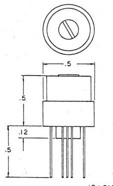
No. **1490 Sensor** may be operated from input voltage of 5 to 20 volts DC with 8 to 13 recommended. Input should be both "spike" and polarity protected. Power requirement is 1 approximately 30 mils (0.030 amps).
