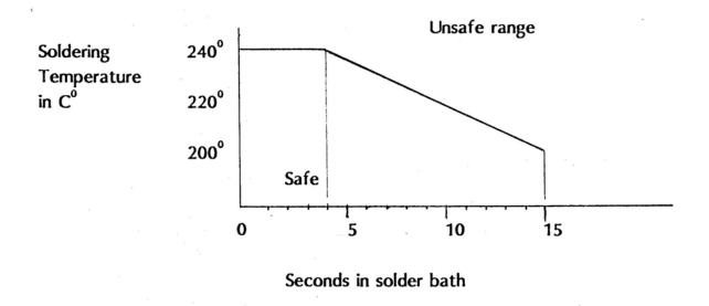
Hand soldering requires particular care for most hand soldering equipment is not accurately temperature controlled.
