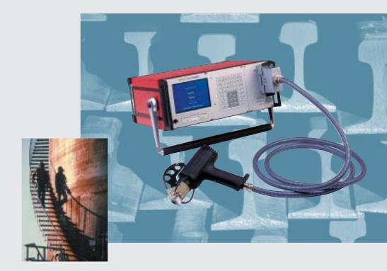
The SPECTROPORT™ provides the portability, flexibility and performance required for modern on-site, metal testing. When true portability is a must, the SPECTROPORT meets the challenge by providing multi-matrix analysis capability in a lightweight and easy to use instrument. The SPECTROPORT can be taken anywhere positive metal identification (PMI) or sorting is required.
