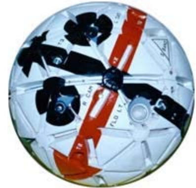
Untethered space robots (conservation of angular momentum is the constraint) (NASA's AERcam)
