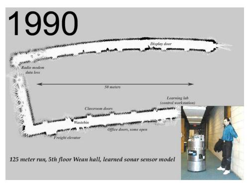
Ten million computations per second and a learned sensor model permitted quite reliable 2D mapping and navigation in real time from sonar range measurements, a performance comparable to the tiniest fish, or a medium insect.
