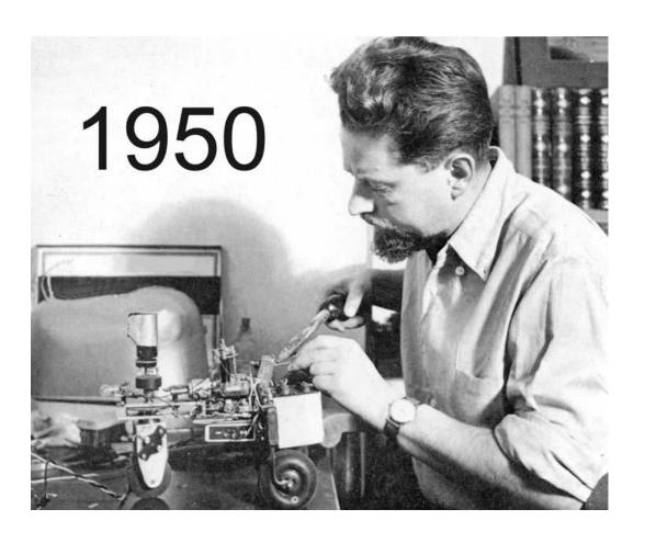
One of eight built, with phototube eye and two vacuum tube amplifiers driving relays that controlled steering and drive motors. Elsie's shell, removed for surgery, can be seen in the background. The tortoises exhibited very lively behavior, for instance dancing near a lighted recharging hutch until their battery ran low, then enter. Their simple tropisms resemble bacterial "intelligence".
