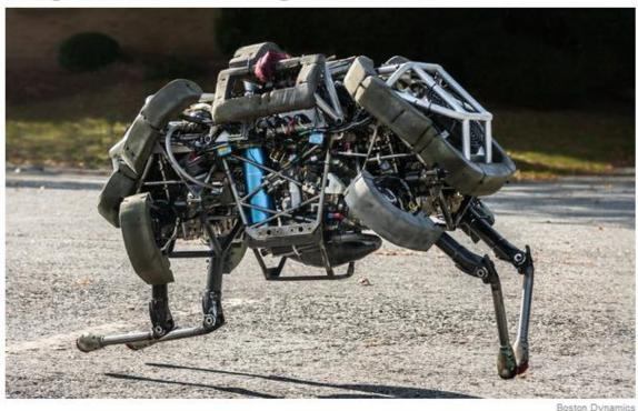
Boston Dynamics' four-legged robot named WildCat can gallop at high speeds.
