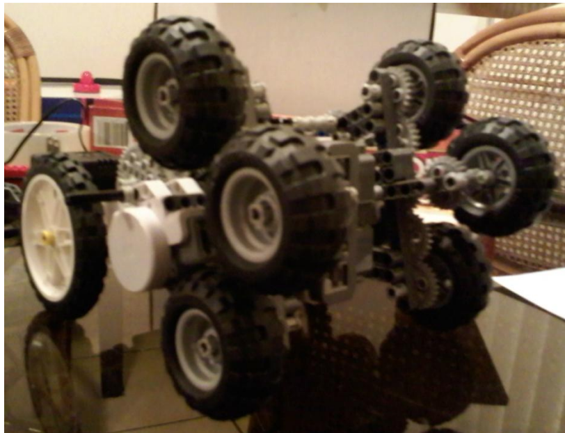
Current prototype. Front view. The vision system will go in between the two front-most wheels
