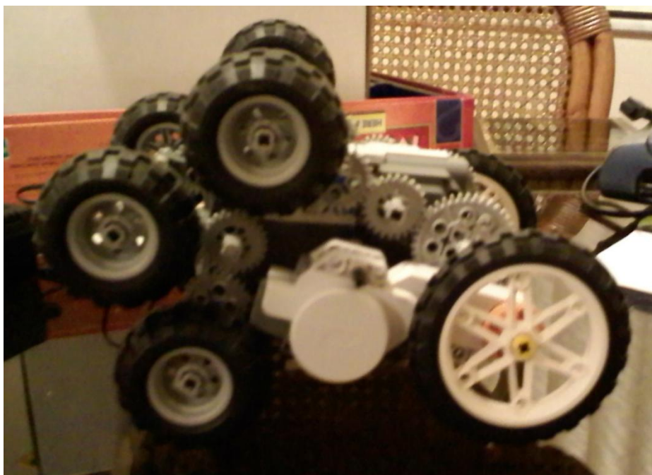
One of the robot's side modules. Notice the 4 wheels, the set of gears, and the NXT motor
