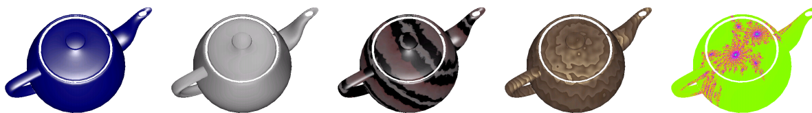
Figure 1: Some images generated by shader metaprograms. From left to right: Phong lighting model, anisotropic satin BRDF via homomorphic factorization, marble and wood implemented using different attributes with the parameterized noise shader, and finally the Julia set (just the texture, no lighting).
