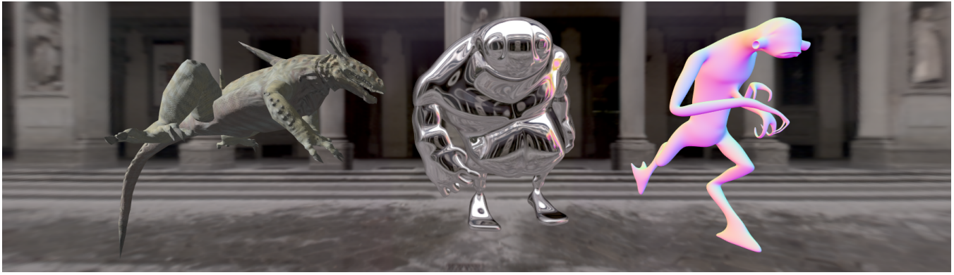
Figure 8: Example models rendered with Spark shaders. From left to right the models are Lizard, Big Guy, and Vortigaunt. Lizard is a triangle mesh with skeletal animation, diffuse/normal maps, and Phong illumination. Big Guy is an approximate subdivision surface rendered with a dynamic reflection cube map (reflecting both the Lizard and Vortigaunt). Vortigaunt uses both skeletal animation and approximate subdivision surfaces. Vortigaunt model data provided courtesy of Valve Corp. Uffizi Gallery light probe image courtesy of Paul Debevec.
