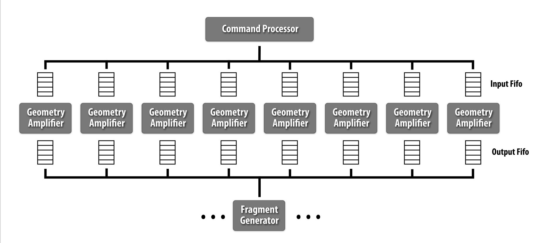
Simple approach 1: make on-chip buffers as big as possible: run fast for low amplification
