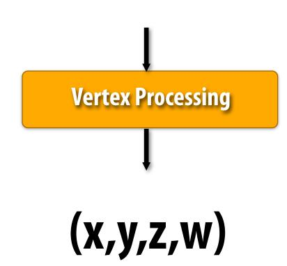
Vertex positions emitted by vertex processing (or the geometry shader, if enabled) are represented in homogeneous clip-space coordinates.
