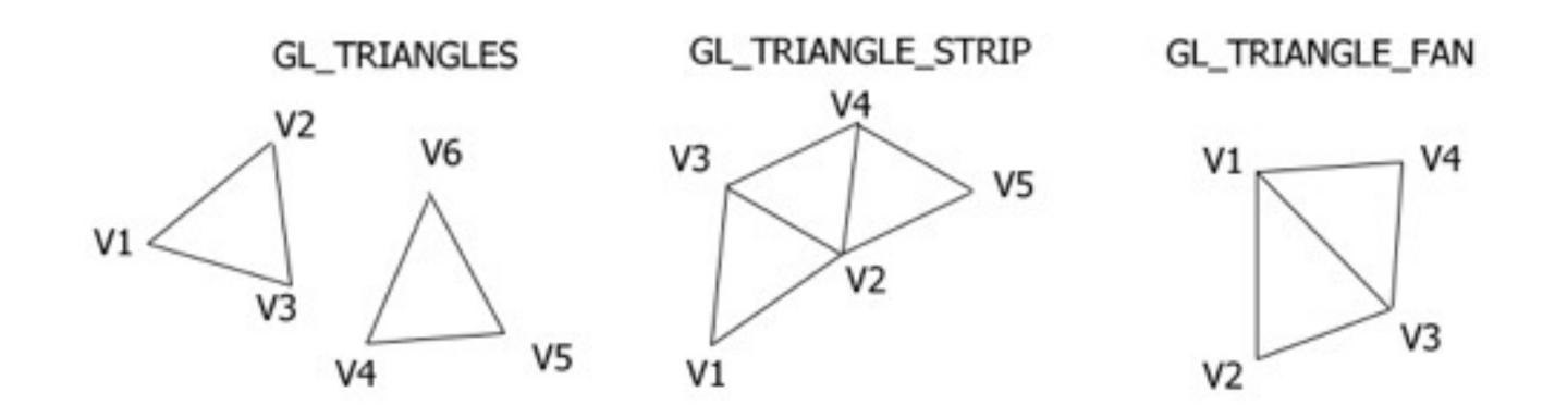
How to assemble is part of graphics state (specified by draw command)
