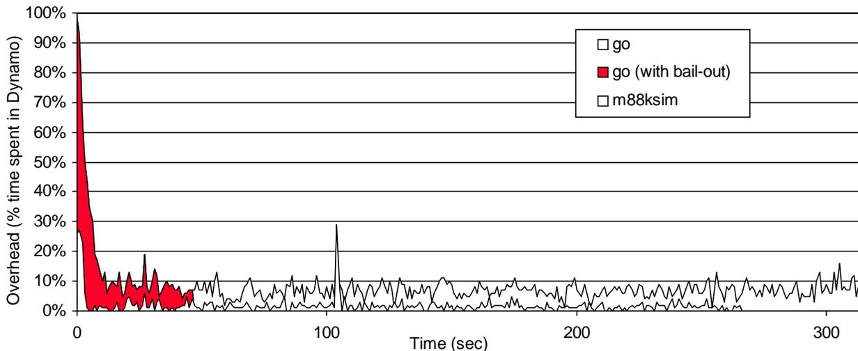
**Figure 8. Illustration of bail-out. Dynamo bails out on *go* ~45 sec into its execution, after which *go* runs directly on the processor without incurring any Dynamo overhead. *m88ksim* is shown for comparison as a case where Dynamo does not bail out.**
