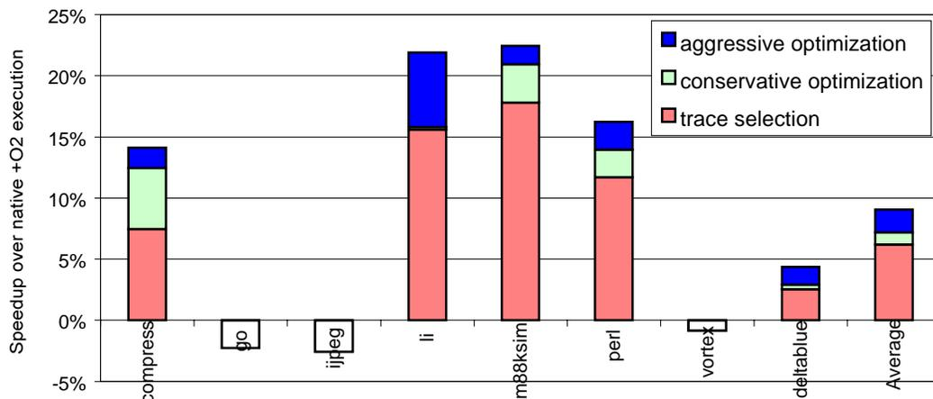
**Figure 7. Speedup of +O2 optimized PA-8000 binaries running on Dynamo, relative to the identical binaries running standalone. The contributions from dynamic inlining due to trace selection, conservative trace optimization and aggressive trace optimization are shown. Dynamo bails out to direct native execution on *go* and *vortex*.**
