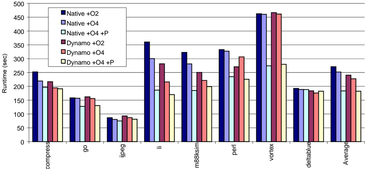
**Figure 8. Dynamo performance on native binaries compiled at higher optimization levels (the first 3 bars for each program correspond to the native runs without Dynamo, and the next 3 bars correspond to the runs on Dynamo)**
