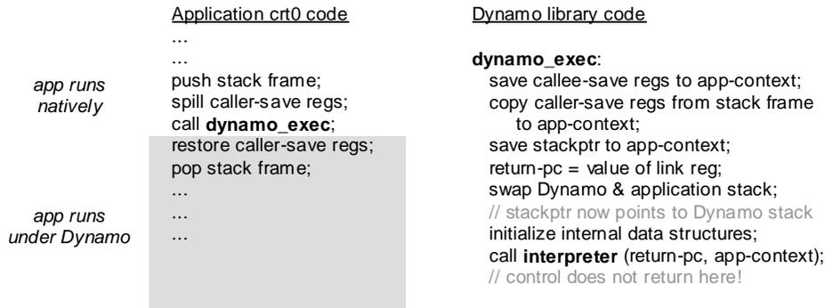
**Figure 2. How Dynamo gains control over the application**
