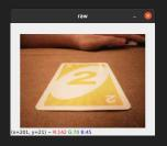
To get around the low contrast on yellow, we stopped looking for light/dark and started looking for yellow/not yellow. Pictured below ('yellow mask') is the result of our color thresholding which spits out a 255 if the color is in the range we called 'yellow', and a 0 otherwise (inverted to match the other pictures). Once we had this nice and crisp, we combined it with the threshold from before to remove the background white.
