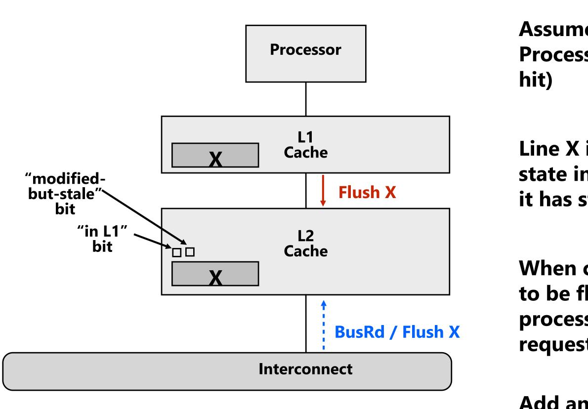
stale" (flushing a "modified-but-stale" L2 line requires getting the real data from L1 first.)
