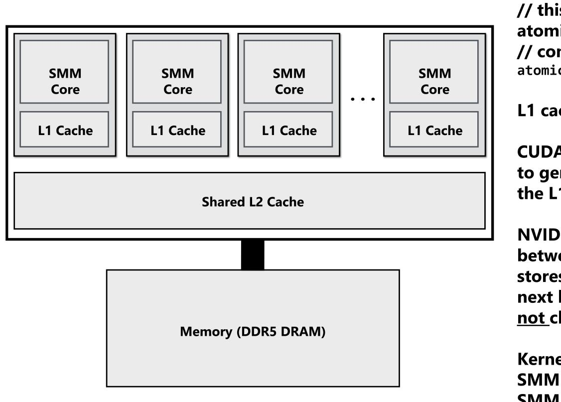
If interested in more details, see "Cache Operators" section of NVIDIA PTX Manual (Section 8.7.6.1 of Parallel Thread Execution ISA Version 4.1) in L2) Kerne
