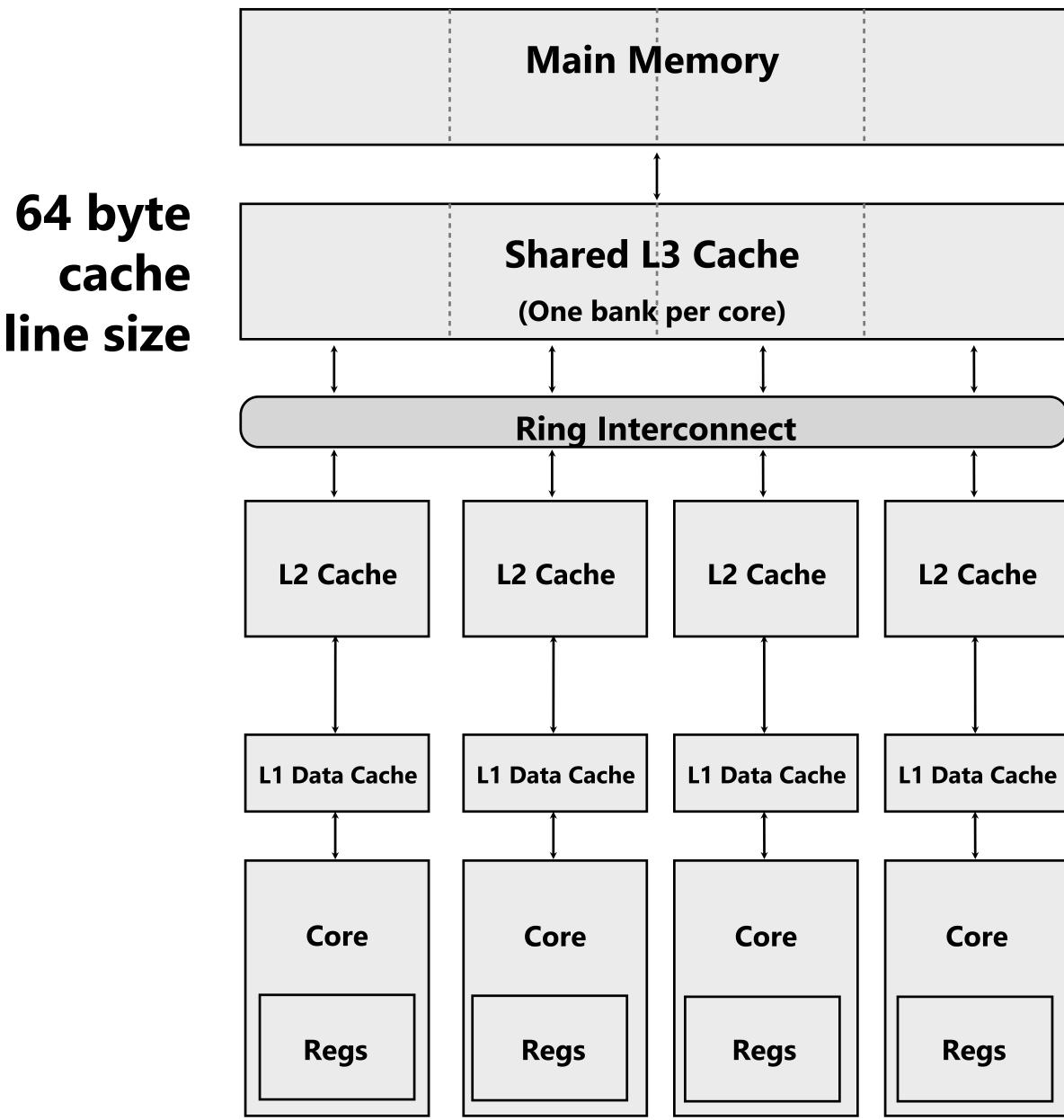
Memory: 2 channels 8 B / channel / memory clock minimum 42 cycles + 51 ns latency
