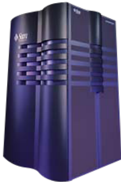
Sun Enterprise 10000 (circa 1997 ) 16 UltraSPARC-II processors
