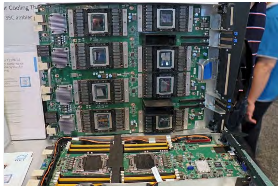
NVIDIA DGX-1: 8 Pascal GPUs connected via high speed NV-Link interconnect
