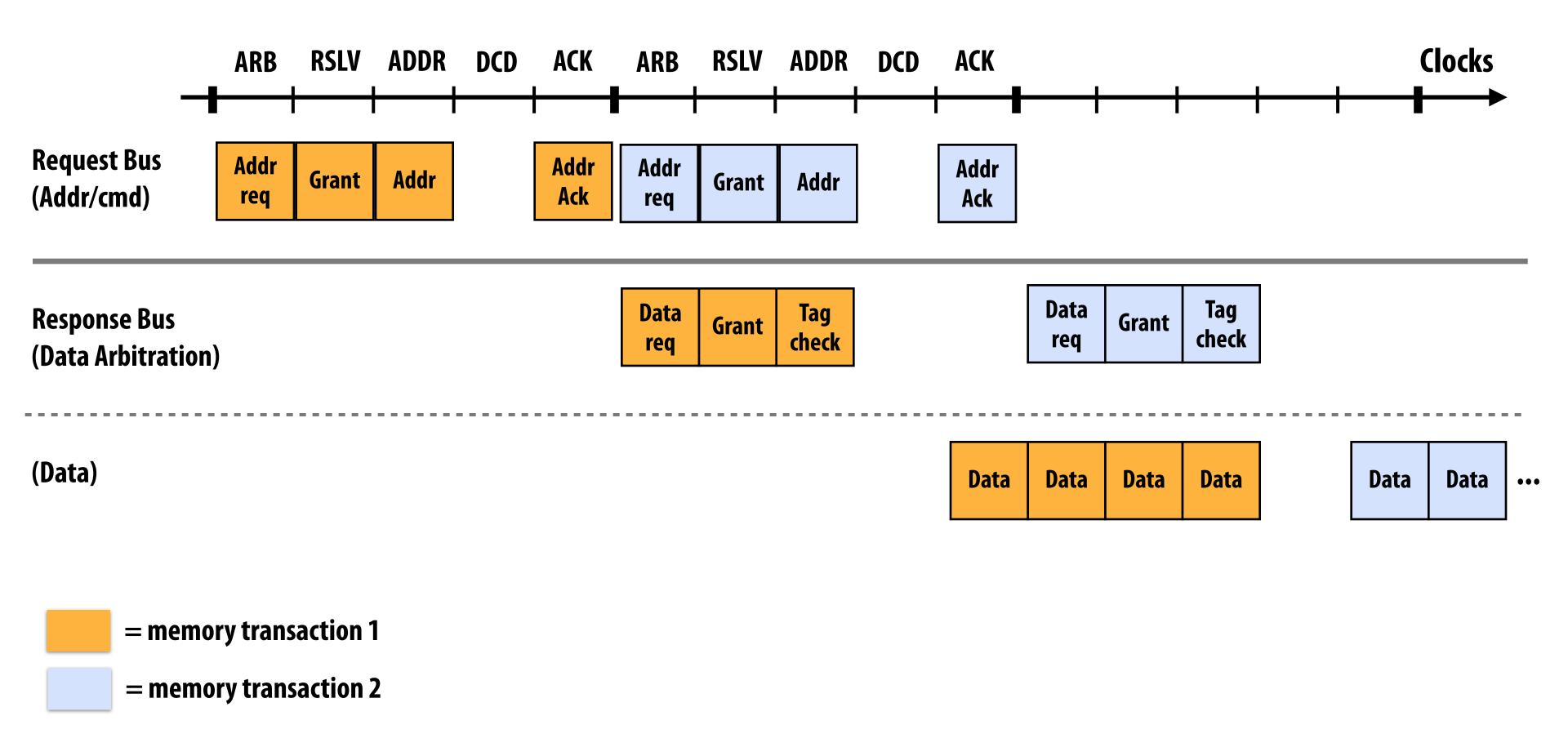
Note: write-backs and BusUpg transactions do not have a response component (write backs acquire access to both request address and data bus as part of the request)
