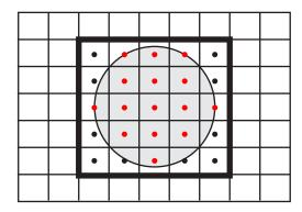
Figure 1: All pixels within the circle's conservative bounding box are tested for coverage. For each pixel in the bounding box, the pixel is classified as covered by the circle if its center point (black dots) is contained within the circle. Pixels centers that are inside the circle are colored red. The circle's contribution to the image will be computed at these pixels.
