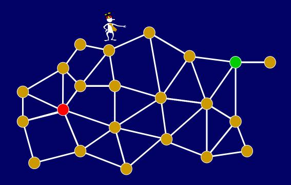
Same as voltage if edges are resistors and we put 1-volt battery between green and red.
