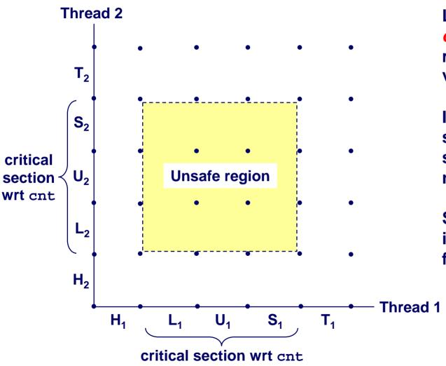
L, U, and S form a critical section with respect to the shared variable cnt.
