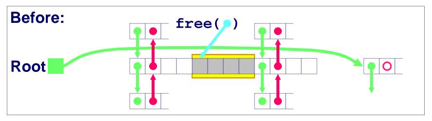
Splice out predecessor and successor blocks, coalesce all 3 memory blocks and insert the new block at the root of the list
