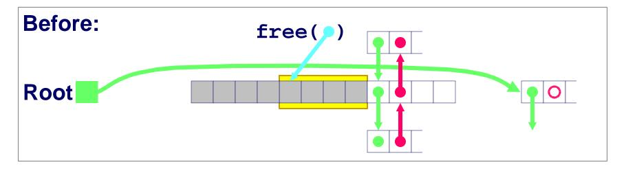
Splice out successor block, coalesce both memory blocks and insert the new block at the root of the list
