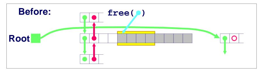
Splice out predecessor block, coalesce both memory blocks, and insert the new block at the root of the list
