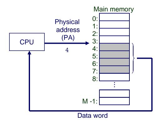
Used by many digital signal processors and embedded microcontrollers in devices like phones and PDAs.
