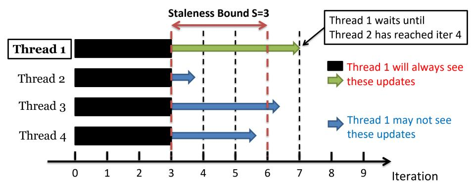
Fastest/slowest threads not allowed to drift >S iterations apart
