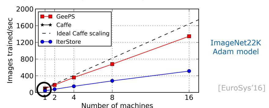
GeePS is 13x faster than Caffe (1 GPU) on 16 machines, 2.6x faster than IterStore (CPU parameter server)
