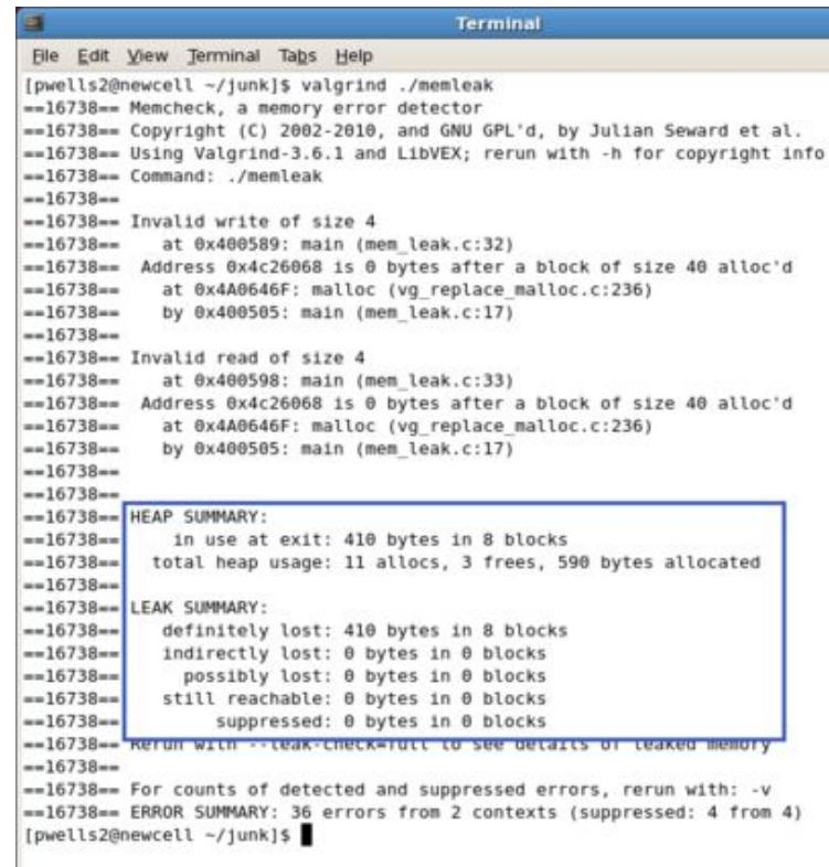
The screenshot shows a terminal window titled "Terminal". The command run is `valgrind ./memleak`. The output is as follows:
