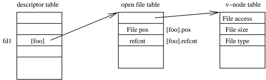
The figure above represents some of the kernel data structures used to manage files. We use  $[x]$  to denote file  $x$ 's descriptor table entry, which points to file  $x$ 's open file table. For example, in the above figure,  $[foo]$  denotes descriptor table entry created in line 6 by the program on the previous page, which points to file  $foo$ 's open file table. Correspondingly,  $[foo].pos$  and  $[foo].refcnt$  denote the “File pos” and “refcnt” entry in its open file table.
