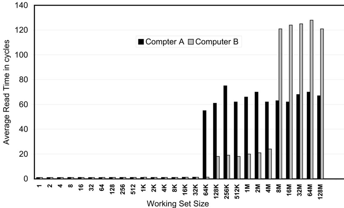
On the vertical axis is the number of cycles for one memory read instruction. The horizontal axis is the size of the test array in bytes.
