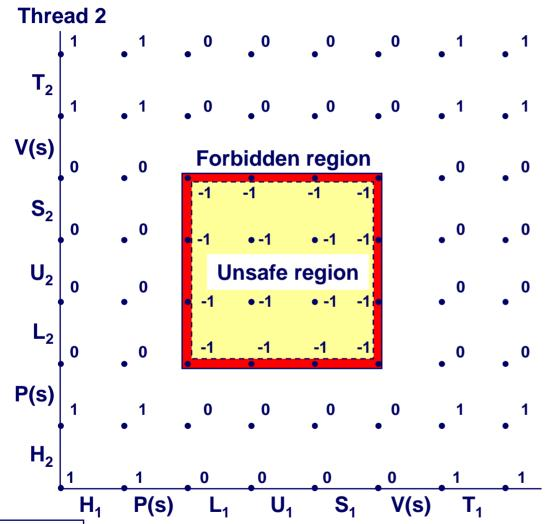
Provide mutually exclusive access to shared variable by surrounding critical section with P and V operations on semaphore s (initially set to 1).
