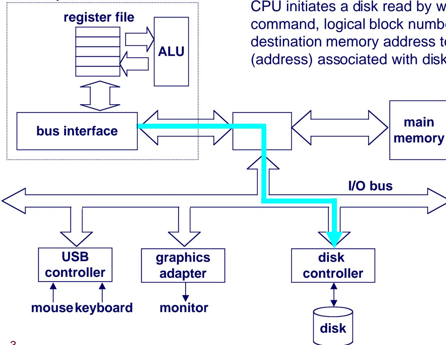
CPU initiates a disk read by writing a command, logical block number, and destination memory address to a port (address) associated with disk controller.
