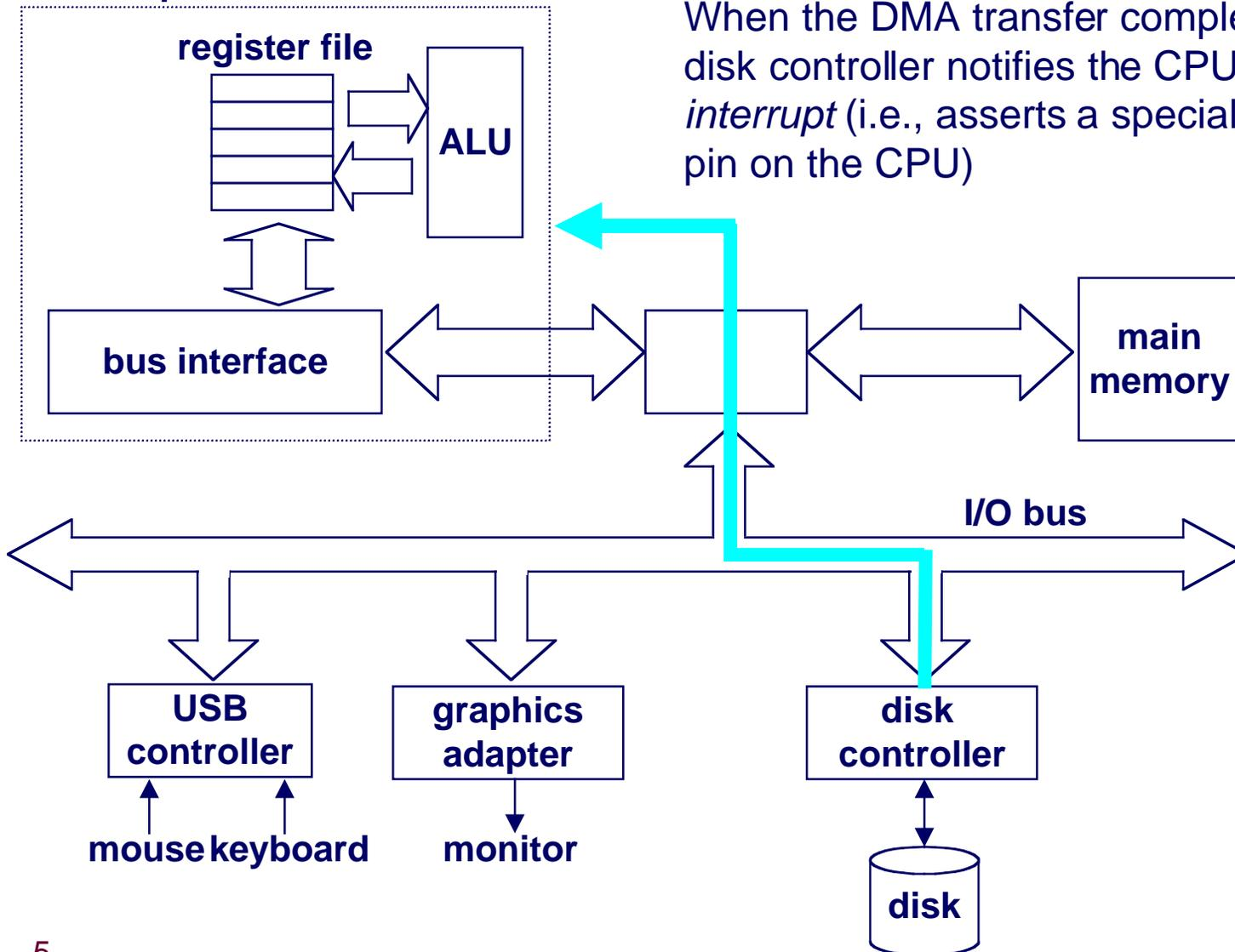
When the DMA transfer completes, the disk controller notifies the CPU with an *interrupt* (i.e., asserts a special “interrupt” pin on the CPU)
