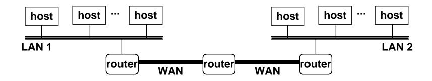
LAN 1 and LAN 2 might be completely different, totally incompatible LANs (e.g., Ethernet and ATM)
