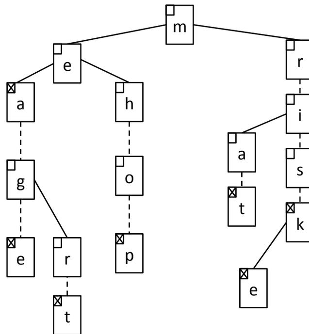
As in the lecture notes, the dotted lines connect a node to its **middle** child, and solid lines connect a node to its **left** and **right** children. An X in the top left indicates that this node ends a valid word. There could be a link to a corresponding value, like a word definition, for example.
