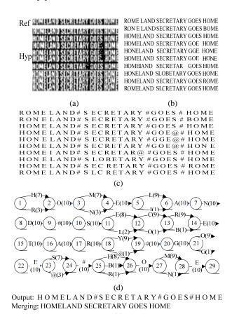
Fig.1 CTN construction. (a) OCR inputs: Text segmentation results; (b) OCR outputs for Ref and Hyp; (c) Preprocessing ("#" for blank, "@" for Null); (d) CTN construction; (e) Decoding for confusion output.
