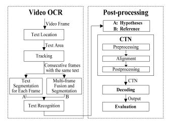
Fig.2 Flowchart of confusion network based framework for Video OCR post processing.
