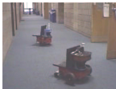
Figure 1: The laser tag robots are equipped with light-emitting devices and receivers.
