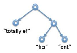
Figure 1: One possible rope representing the string "totally efficient".
