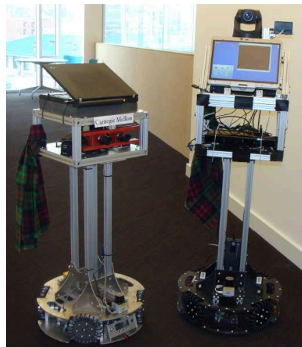
Fig. 1: The CoBot mobile service robots. CoBot robots autonomously perform tasks in human-populated environments, often without any supervision. This makes robustness during navigation a particularly relevant problem.
